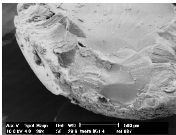
Fig. 2. Sliced bead, showing amorphous core and crystalline surface, following exposure to ethanol/water vapour in the IM.
